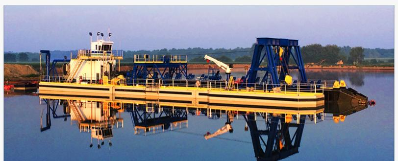
A Cutter Suction Dredge manufactured by Custom Dredge Works
